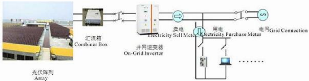
电站系统图Roof-Top PV System
